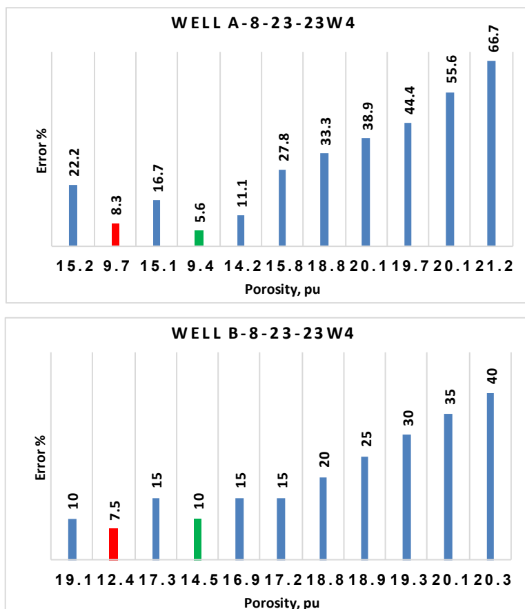
Figure 7: The sum of all mistakes made when trying to calculate the net pay of the chosen wells in the dataset. The Jensen and Menke method of cut-off is shown in green, whereas the conventional way is shown in red
