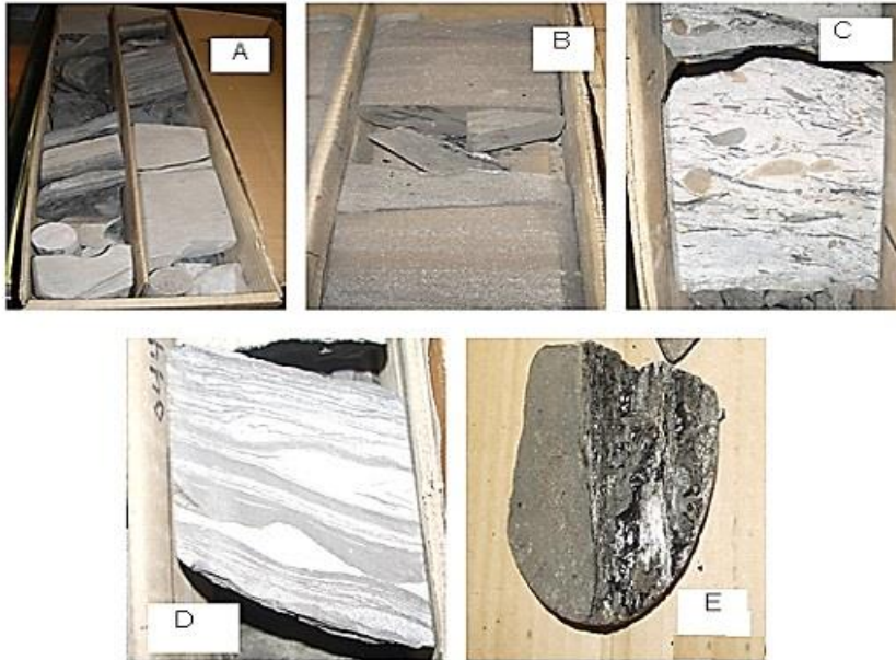
Figure 4: Cores from study wells. A. Gray fine-to-lower medium grain size, and low-angle cross-bedded sandstone of well B-8-23-23W4. B. Siderite (Brownish color). Siderites are abundant in both cores. C. 10 cm piece of upper fine to lower medium sand with mudstone-clasts conglomerate, carbonaceous, chert at the well A-8-23-23W4. D. Wavy, low-angle alternative shale, and sand bed, with 2-10 mm in thickness. E. Coal clasts of the well B-8-23-23W4
